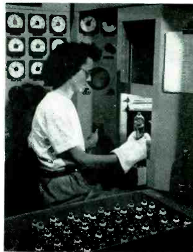
Mercury and gas-filled tubes are tested in 30 seconds by the recently developed machine shown
