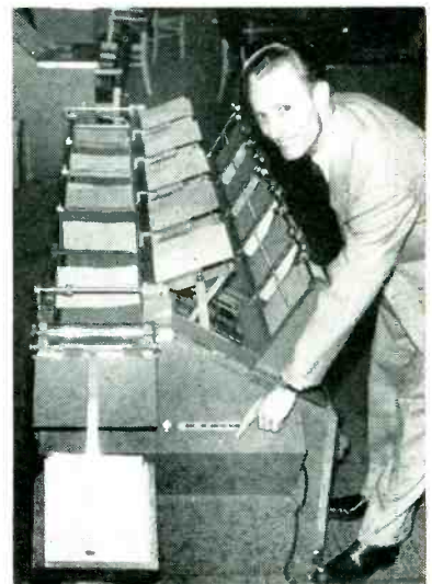
High-speed collator's accuracy is assured by electronic controls which supervise its operation
