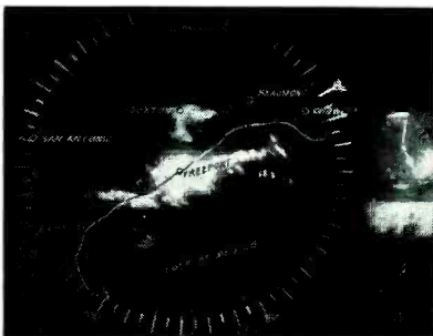
Radar ppi scope picture of line squall at Freeport, with geographical features dubbed in
