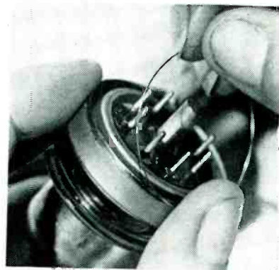
Copper-gold brazing alloy being placed around base of tube prior to brazing operation
