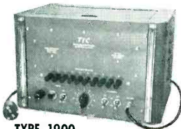
TYPE 1900 CRYSTAL CONTROLLED MULTI-FREQUENCY GENERATOR
