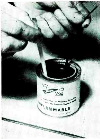
New magnetic fluid makes residual magnetic field visible when recorded tape is dunked as shown. Resulting pattern appears after about one minute of drying in air, as on two-track recorded tape sample on table. Powder can be wiped off without damaging tape
