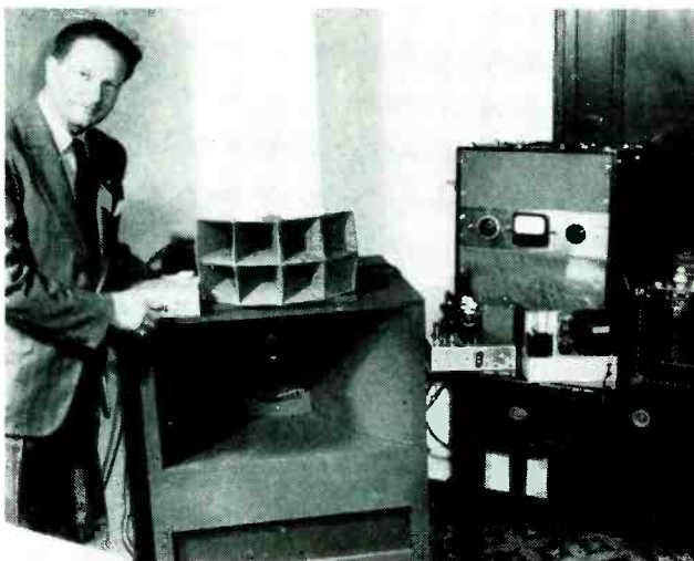
Corner of Peerless Electrical Products Division's exhibit room, with H. M. Morris adjusting tone control unit of musician's sound system. Sound source is magnetic tape recorded off the air; amplifier (on table) uses Williamson circuit developed in England, with Peerless transformers; speaker is Altec 800, theater unit
