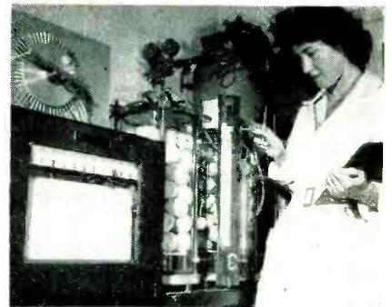
Lemon life in storage can be prolonged by checking fruit regularly with this special oxygen analyzer and recorder, which determines whether breathing is at a healthy rate
