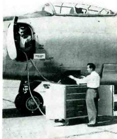
North American engineers check a B-45's radar equipment with their recently-developed continuity and megger checker
